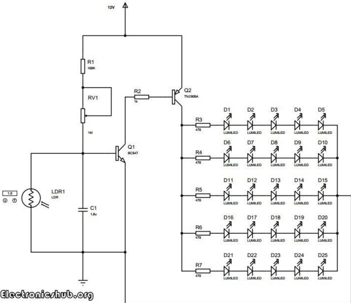
The transistors are used in saturation mode. They are used as electronic switches in this mode. The transistor BC547 is a general purpose NPN transistor which is used to further switch the LEDs. This is a power transistor with a heat sink. The heat sink helps the transistor to dissipate the generated heat into air so that the transistor can handle higher power loads than it can do without the heat sink.
